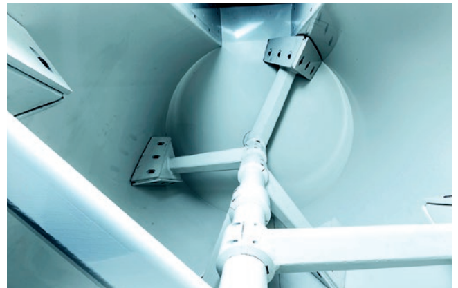
Mixing unit with dual rotation paddles
